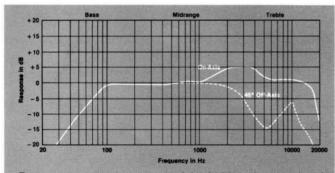
Frequency response contour of the 8130H taken in a hemispherical free-field environment. Measured response of a typical production unit, including all peaks and dips, does not deviate more than 4 dB from the above curve. Additional acoustic loading will further extend bass response.
