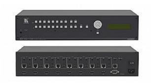
The VS-88DT is an HDMI/HDBT matrix switcher for HDMI, HDBaseT and IR signals. The unit accepts up to eight HDMI and IR inputs and routes any or all of them to any or all of eight HDMI or HDBaseT and IR outputs for connection to compatible HDBaseT receivers, for example, the TP-580RXR.
