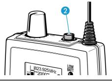
The ground connection of the earphones cable serves as the antenna for the second diversity section. For details on the connector assignment, refer to the diagram on page 26.
