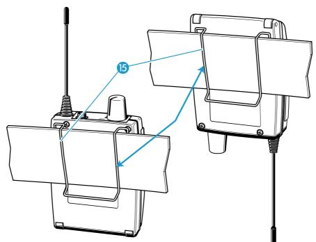
The belt clip is detachable so that you can also attach the diversity receiver with the antenna pointing downwards. To do so, withdraw the belt clip from its fixing points and attach it the other way round. The belt clip is secured so that it cannot slide out of its fixing points accidentally. To detach the belt clip:
