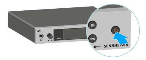
To switch the receiver to standby mode:
