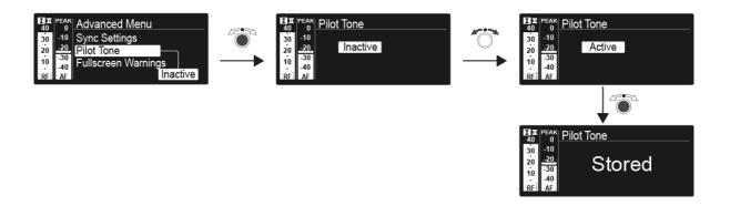
The pilot tone has an inaudible frequency that is sent from the transmitter and evaluated by the receiver. It supports the receiver's squelch function.
