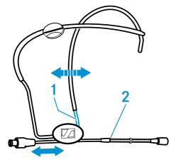
If necessary, precisely position the microphone by using the flexible gooseneck 3.
