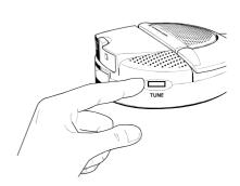
TUNE button on the earpiece and the auto-tune function will re-tune to the next strong signal. Repeat this until you can hear the audio signal loud and clear. If you decide to change the transmitter channel, the receiver search tuning must be restarted by pressing the TUNE button on the headphones again.
