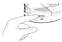
because of interference or another nearby system), press the TUNE button on the earpiece and the auto-tune function will re-tune to the next strong signal. Repeat this until you can hear the audio signal loud and clear. If you decide to change the transmitter channel, the receiver search tuning must be re-started by pressing the TUNE button on the headphones again.
