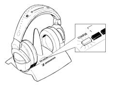
the transmitter, the one next to the "charge" light). The red LED on the transmitter must light up to show charging is taking place.
