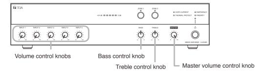
The unit's volume level can be adjusted in 2 steps using individual input volume control knobs and the Master volume control knob. Therefore, when the Master volume control knob is set to the minimum position, no sound is output even if each input volume control knob is set to the maximum. Be sure to adjust the entire volume level with the Master volume control knob in advance.
