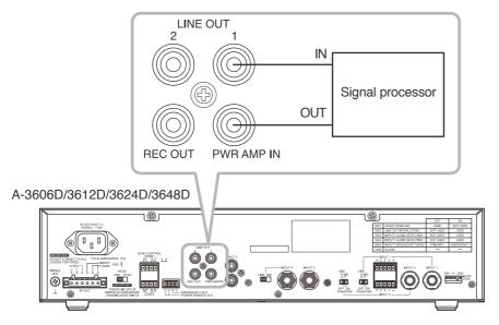
Line output specifications:  $0 \text{ dB}^*$ , 600  $\Omega$ , unbalanced, RCA pin jack Power amplifier input specifications:  $0 \text{ dB}^*$ , 600  $\Omega$ , unbalanced, RCA pin jack
