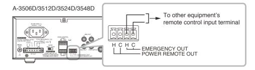
Output specifications: Open collector output, withstand voltage: 30 V DC or less, current: 25 mA or less
