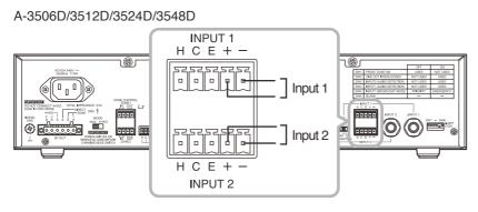
Input signal specifications: Short-circuit current: 10 mA or less, open voltage: 35 V DC or less
