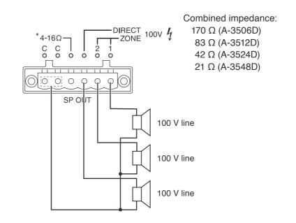
For the audio output at high impedance application setting, refer to "21. Speaker output terminal" on p. 9.
