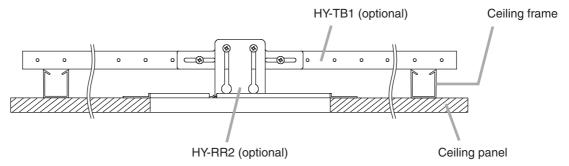
2-3. Ceiling mounting in a larger than specified hole
