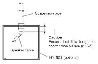
Step 3. Connect the speaker cable to the push-in terminal.
