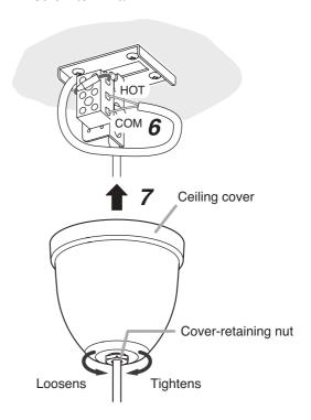
Step 7. Push the ceiling cover, slipped over the connected cables, onto the ceiling surface, then tighten the cover-retaining nut using a 17 mm (0.67") hex wrench.
