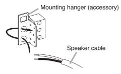
**Step 4.** Connect the speaker cable to the screw terminal.
