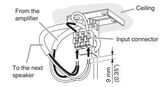
**Step 6.** Push the ceiling cover, slipped over the cord in Step 2, onto the ceiling surface, then tighten the cover-retaining nut using a 17 mm (0.67") hex wrench. In the case of exposed wiring, notch the cable entry tab on the rim of the cover, then make connections.
