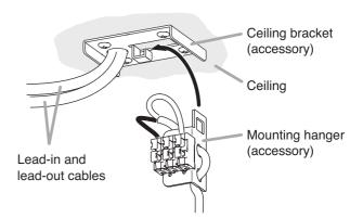
**Step 5.** Connect both the lead-in and lead-out cables to the input connector.
