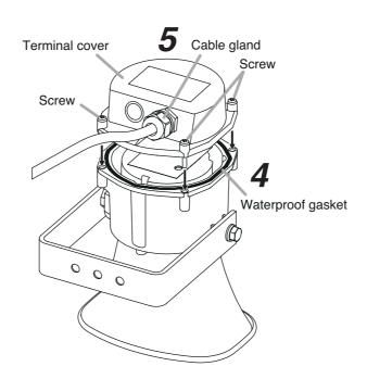
Step 5. Securely tighten the cable gland.
