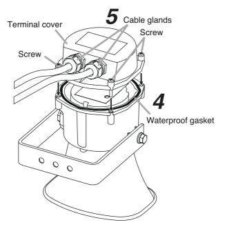
Step 7. Securely tighten the cable glands.
