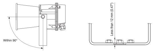
• Do not install the speaker face-up from a horizontal plane. If water accumulates in the horn, this may cause the speaker malfunction.
